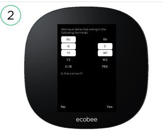
Ensure that Rc, G,  $Y_1$ , C, and  $W_1$  are the only wiring terminals highlighted and tap "Yes."
